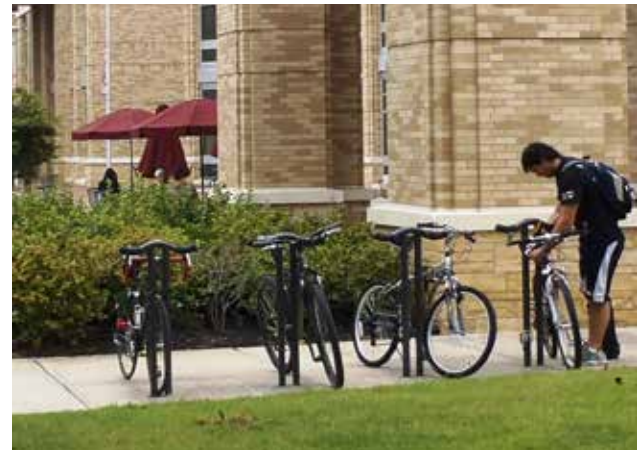
The "Pi" style bike rack offers flexibility in location and quantity of racks.
